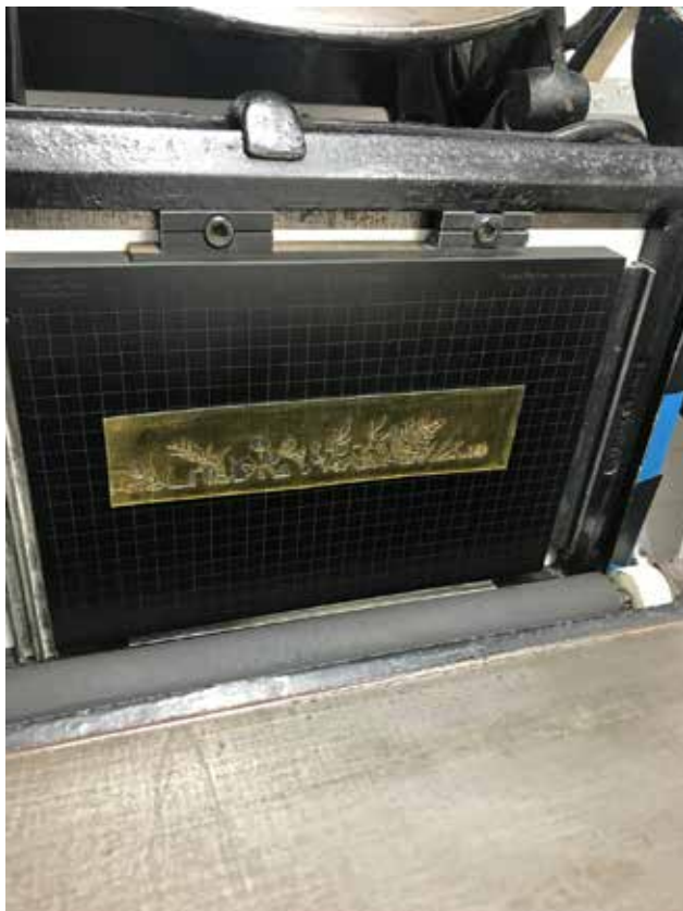
Pic 2. Showing the position of the Female Polymer plate on the press.
